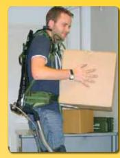
advantages of exoskeletons is the ability to remove the heavy load on a worker's torso, thus greatly reducing the injurious forces
