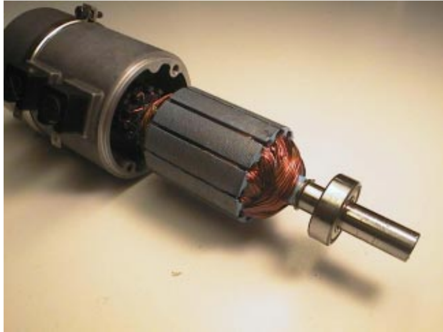
Figure 3: Coils of copper run lengthwise along the rotor and are called armature windings. These are responsible for carrying the current through the magnetic field of the stator.
