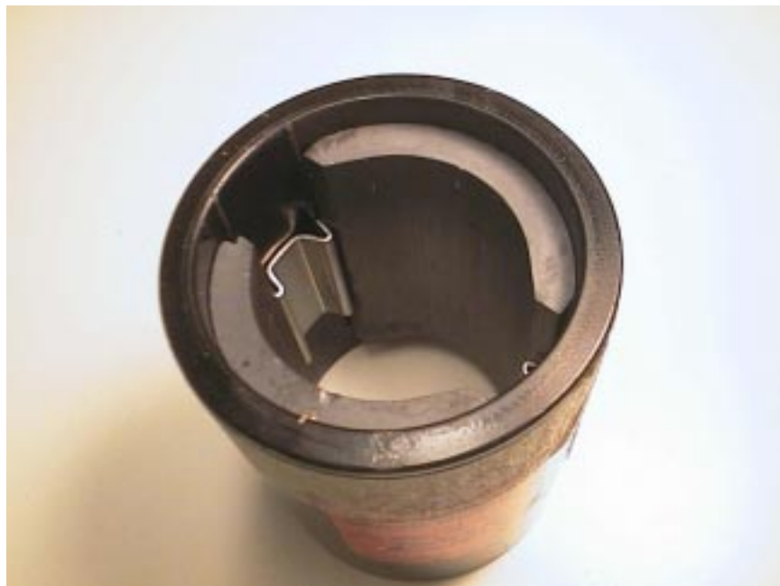
Figure 2: Permanent magnet stator. The two pieces establish a magnetic field.
